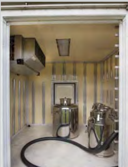
Milk vats in a refrigerated van that pulls the mobile milking unit.
